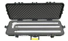
Pictured above is an example of our stingers we use to offload products with a specialized air pump. Pictured below is a prop we can use to cold tap (drill a hole in a semi-trailer to gain access to liquids) and unload the product into an undamaged trailer. The round disc on the bottom right is made of the same material as a trailer and we use hole saws and drills to cut holes for access to put the stinger in.
